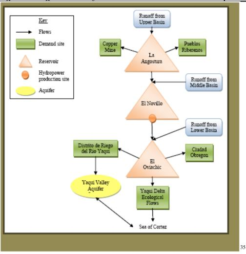
Figure 2: Diagram of the Hydro-electric dams north of the Rio Yaqui territory
